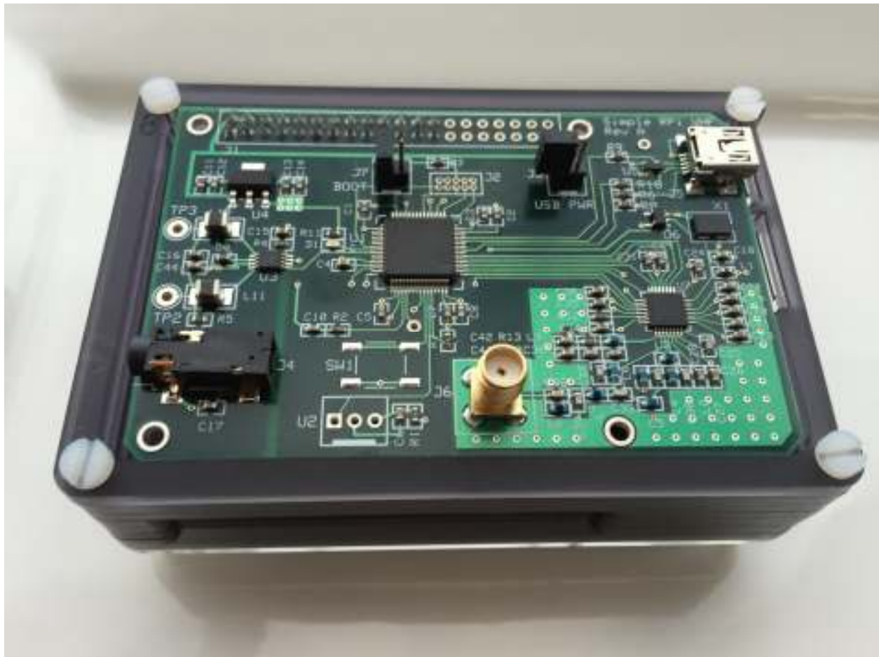
Figure 1: The complete transceiver and TNC fits on a 3.35 by 2.2 inch printed circuit board.
